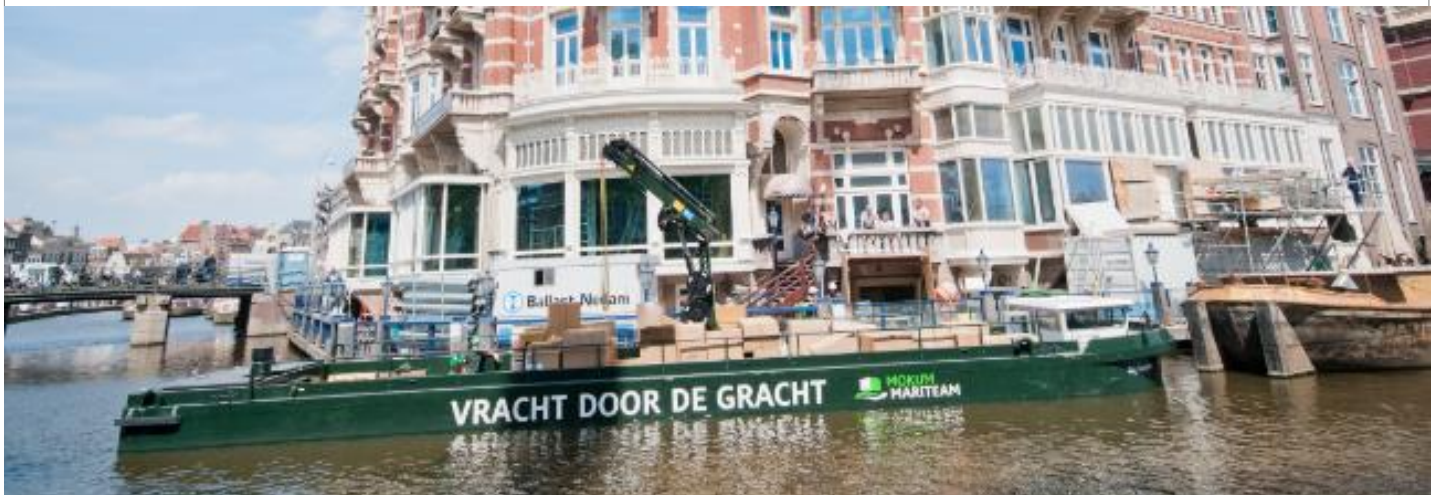
Mokum Mariteam full-electric barge with own crane, operating in Amsterdam 20 m length, 4.25 m width, 85 m 3 load capacity
